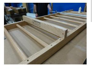
7. Orient the Logo on the front of the backer board correctly at the top of the unit. Drill pilot holes using 1/8" drill bit. Use 2" screws and secure the 2 mounting brackets to the back of the side rails.
