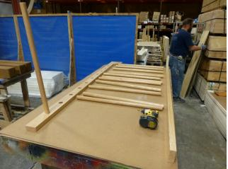
2. Lay out 8' side rails parallel to each other about 3ft apart. Lay out all 12 rungs and line them up with the side rail holes.
