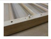
6. Working on the back of the unit place the 4 small wood dowels and glue in the proper holes on the back of the side rails and place the 34" mounting bracket on the dowels using their predrilled holes. Secure the unit firmly with the 42" pipe clamp. Be sure to protect the wood from damage from the clamp.
