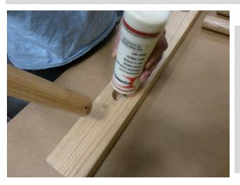
3. Apply a layer of wood glue in the hole and firmly press the rungs in the hole until they are seated in the bottom of the hole. Notice the pre-drilled holes in the rungs and twist the rung to align them with the small holes in the side rails so they are ready to accept the 3" screws. Clean any glue that may have spilled from the hole.
