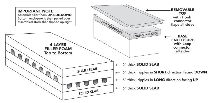
This product is shipped unassembled to reduce freight cost, as well as reduce the possibility of shipping damage. Assembly is easy and will acquaint you with interchangeable filler feature. Supplied components are as illustrated above.
